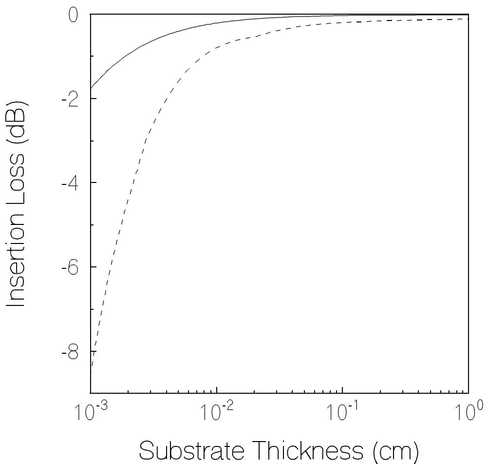
**Figure 2** Calculated insertion loss as a function of the ferrite substrate thickness for a circulator junction (solid line) and for a circulator junction plus a network transformer (dashed line).
