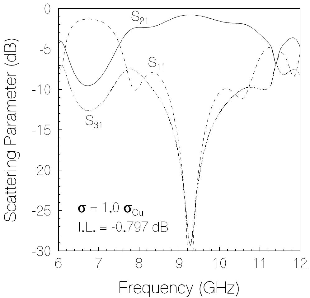
**Figure 1** Calculated S-parameters of a thin-film circulator connected to a impedance transformer network. The substrate thickness is 100  $\mu\text{m}$ .
